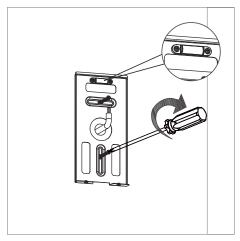
Fix the mounting bracket onto the wall by screws (gradienter to ensure the level)
