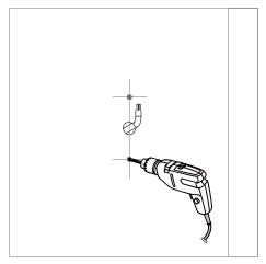
3. Drill two holes on the wall (Φ=8mm, depth=50mm, distance 85-125mm)
