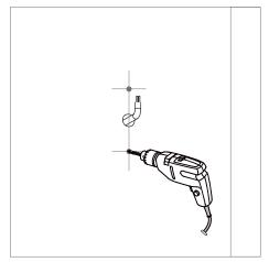
2. Drill two holes on the wall (Φ=8mm, depth=50mm, distance 85-125mm)
